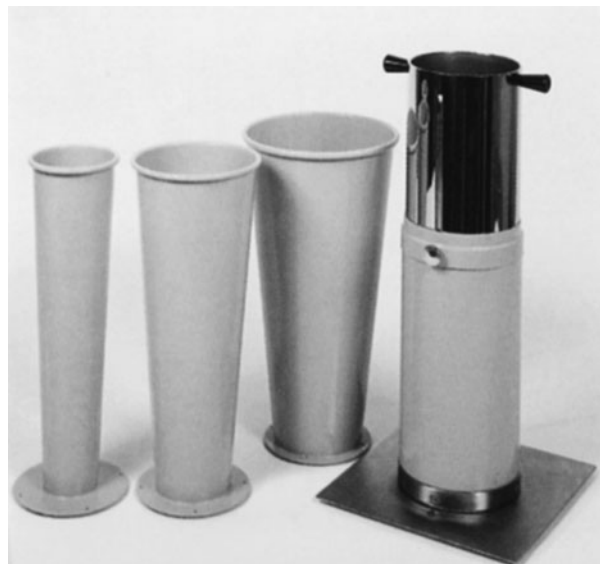
Figure 8-1. Cylinder cones (especially the extendible type) are generally considered more efficient than aperture diaphragms because they restrict the size and shape of the x-ray beam for a greater distance. The closer the distal end of the beam restrictor is to the area of interest, the greater its efficiency. (Courtesy of Burkhart Roentgen, Inc.)
