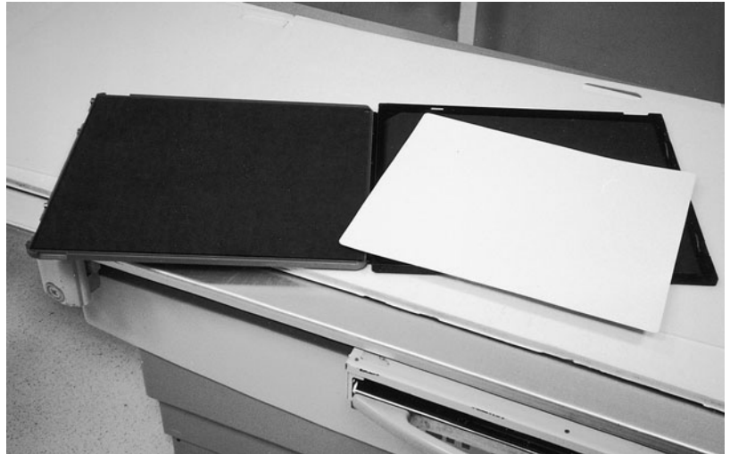
Figure 12–5. A CR cassette is very similar in appearance to a conventional screen–film cassette. The CR cassette holds an image plate (the image receptor) between its front and rear panels. There is no film or intensifying screens. (Reproduced, with permission, from Shephard CT. Radiographic Image Production and Manipulation . New York: McGraw-Hill, 2003).
