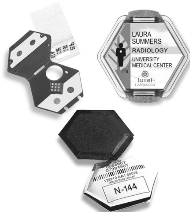
Figure 10–1. OSL dosimeters are available with various combinations of filters. Some contain a filter pack of tin, copper, and an open window. Others are available with aluminum, copper/aluminum, plastic, and an open window. Still others contain lead, copper/aluminum, plastic, and an open window. These various filters serve to identify the type and energy of radiation. (Courtesy of Landauer Inc, Glenwood, IL.)
