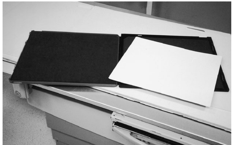
Figure 11–67. A CR cassette is very similar in appearance to a conventional screen/film cassette. The CR cassette holds an image plate (the image receptor) between its front and rear panels. There is no film or intensifying screen. (Reproduced, with permission, from Shephard CT. Radiographic Image Production and Manipulation . New York: McGraw-Hill, 2003).
