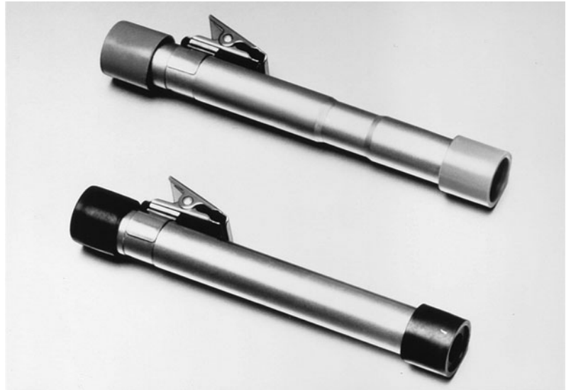
Figure 10–4. The pocket dosimeter contains a small ionization chamber that counts charges in proportion to the exposure received. (Courtesy of Nuclear Associates.)
