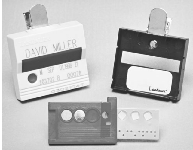
Figure 10–3. The thermoluminescent dosimeter (TLD) contains crystalline chips of lithium fluoride (LiF), which absorb and store the energy associated with exposure to ionizing radiation. (Courtesy of Landauer Inc, Glenwood, IL.)
