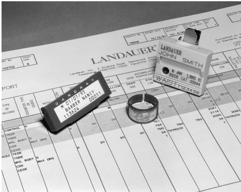
Figure 10–6. The film badge ( left ) contains filters to determine the type and energy of radiation received by the wearer. The TLD ( right ) contains thermoluminescent crystals that emit quantities of light proportional to their degree of exposure. The ring badge ( center ) is particularly useful for individuals whose hands are in close proximity to radioactive nuclides or the fluoroscopic x-ray field. A report similar to the one shown is returned monthly, documenting the radiation dose received by each of the personal monitors. (Courtesy of Landauer Inc, Glenwood, IL.)
