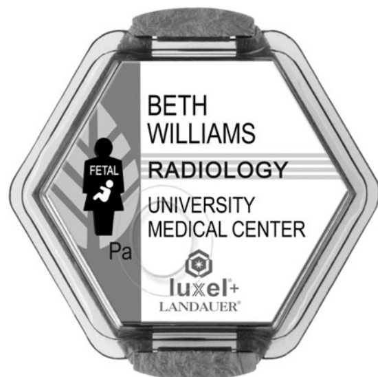
Figure 10–5. The pregnant radiographer should wear a second, waist-level, dosimeter under her lead apron that will measure approximate fetal dose. (Courtesy of Landauer Inc, Glenwood, IL.)
