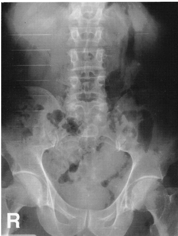
Figure 13–40. Minus-density artifacts (scratches), running in the direction of film travel, caused by misaligned guide shoes.
