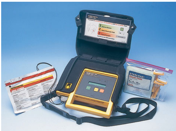
FIGURE 5.27 An automated external defibrillator (AED) is designed for use by nonprofessionals in emergency situations when defibrillation is required.
